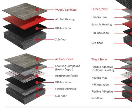
1: The sub-floor, whether concrete or wood, should be made suitable for the chosen floor covering (ie tiles) prior to any boards being fitted. The boards are designed to provide increased insulation levels not structural rigidity.
