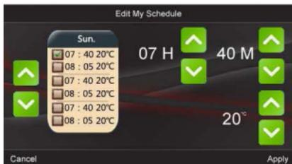
In each column there is 6 periods / zones. The time for each zone should be set in consecutive times throughout the day i.e. 7 – 8 – 9 – 10 etc. and not 7 – 10 – 8 – 9 etc. The temperature set for each time zone will be held by the thermostat until the next time zone starts. H = Hours, M = Minutes and bottom right number is set temperature. Once all times and temperatures are set simply press “APPLY” to save the new schedule settings.
